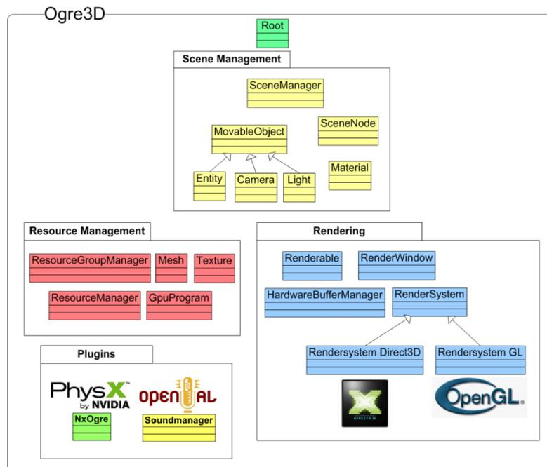
Figure 3. Ogre3D – graphic-engine with physics and sound plugins
