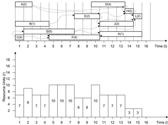
Figure 2. Resource levelling of the example network using the Minimum Moment Method.
