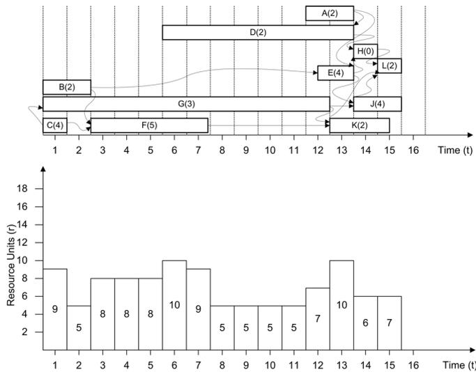
Figure 3. Resource levelling of the example network using the Entropy Maximization Method.
