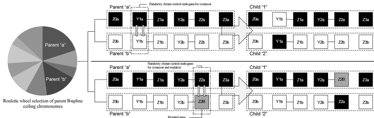
Figure 2: Process of evolution through parent selection, crossover and mutation.
