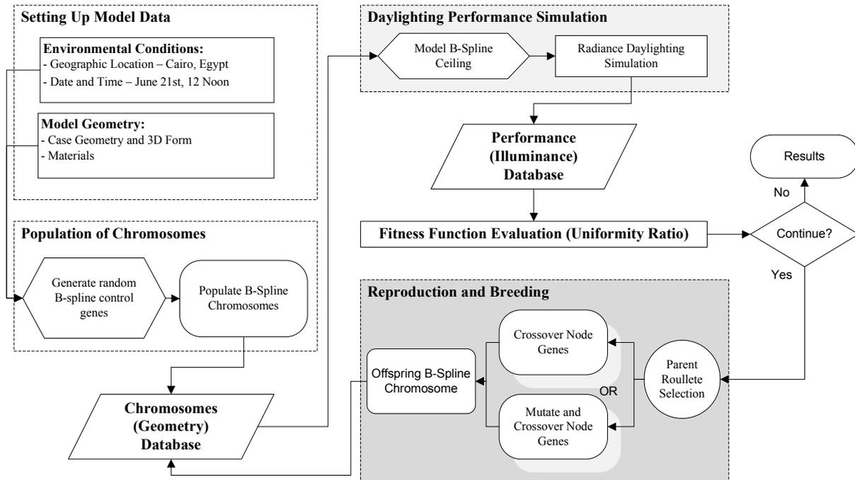
Figure 3: Schematic of GA process integrated with B-Spline ceiling form finding.
