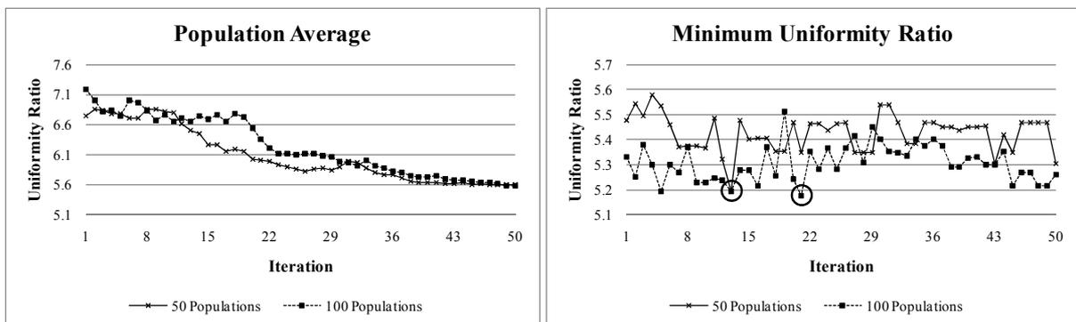
Figure 6: Iteration against uniformity ratios. Showing minimum uniformity ratios and population averages.
