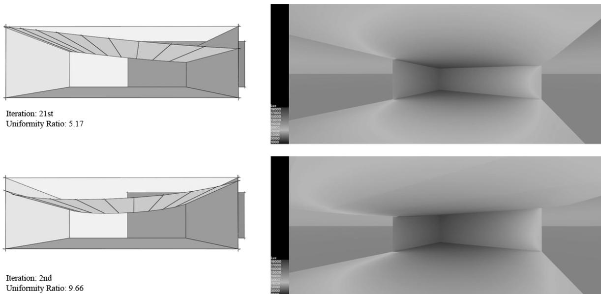
Figure 8: Best and worse solution geometry, with false colour rendering (100 p/i).
