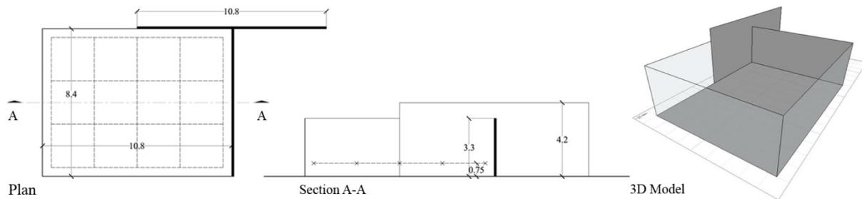
Figure 4: Assumed design parameters of the analyzed indoor space.
