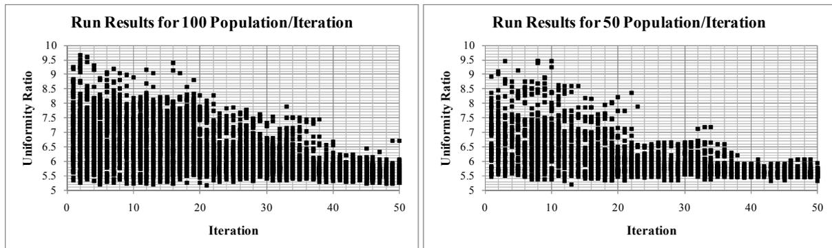
Figure 5: Iteration against uniformity ratios, GA runs results.
