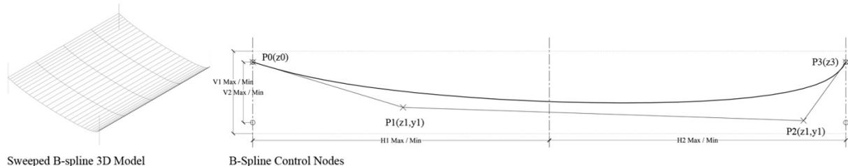
Figure 1: Example cubic B-spline ceiling with four control points (P0, P1, P2 and P3).
