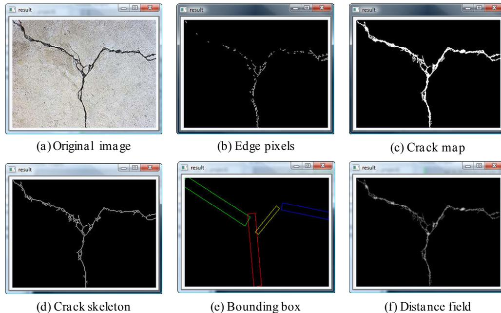
Figure 3: Immediate and final results of the method; the crack is divided into four segments based on the orientation information (S1-red, S2-green, S3-blue and S4-yellow).
